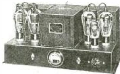
Fig. A, below. The extreme compactness and neatness of this 100-watt power stage, also layout, are clearly shown.
